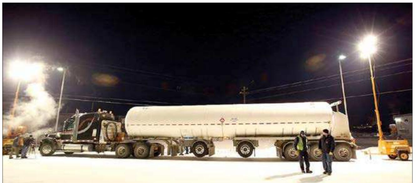
A specially designed trailer to transport supercooled liquefied natural gas is seen on display in front of the Fairbanks Pipeline Training Center. The Alaska Industrial Development and Export Authority and Fairbanks Natural Gas are evaluating the new trailer.
